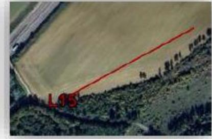
Unit Electrode Spacing = 2.50 m.
